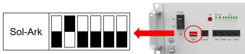
Figure 2.1.1.4 Sol-Ark inverter DIP Switch Setting
