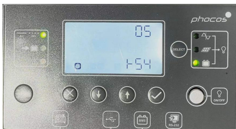
Figure 2.1.2.5 Phocos inverter battery type selection
