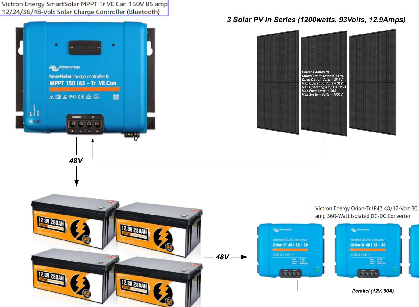
4, 12V 280AH, LifePO4 Batteries with integrated BMS in Series (48V)
