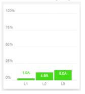
Shows reported current per phase wire. The graphical presentation is scaled according to setting of Configuration/Meter/Main fuse.
