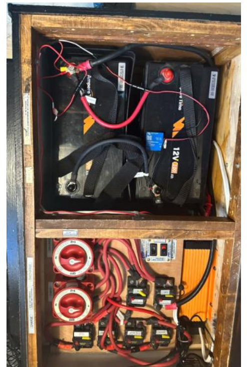
Even broader view including Bank 1, 200 lithium amp hours (total 400 with both banks)
