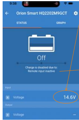
Step 3) Confirm voltage is coming into DC Charger
