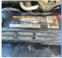
Step 1) Car battery. When OFF Voltage is 12.5V When ON Voltage is 14.5
