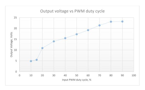
I have measured the output voltage as the function of the input PWM duty cycle, and as you can see **the retrofit kit works as it should work.**
