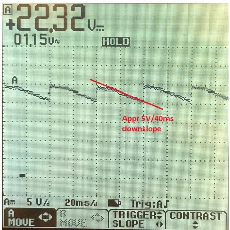
A simple formula dU/dt = I/C gives the value of the capacitance about  $100\mu F$ . This capacitor at the output of the fan controlling stage makes it impossible for the retrofit kit to work correctly, because the retrofit kit needs to "see" full amplitude of the 25 Hz PWM signal.
