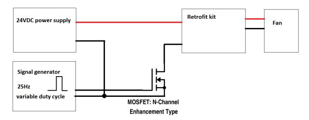
I do not have a Multiplus device build before HQ2224, and I have assumed that its output stage, controlling the fan, should consist of a simple top-side or bottom-side Mosfet.
