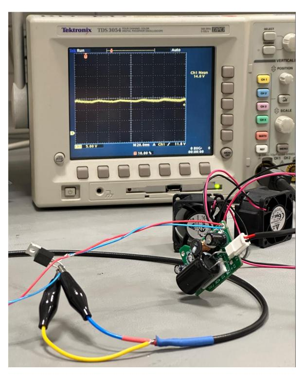
By changing the duty cycle of my signal generator, I can simulate the behavior of the PWM output stage at 25Hz and different requested cooling capacities.
