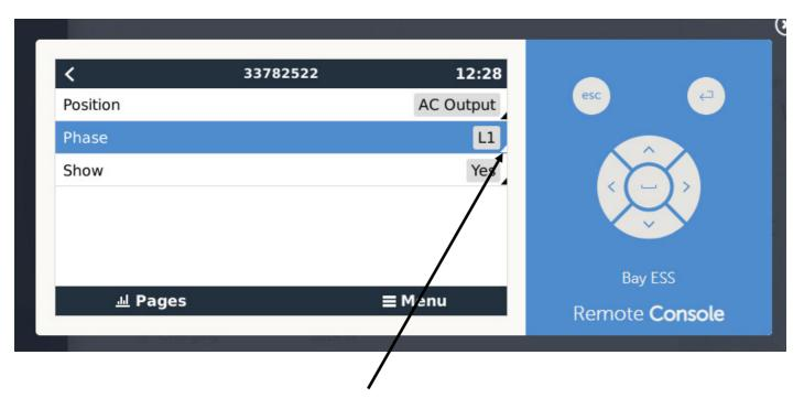
This little triangle was not there, it was Reading "MultiPhase" and we couldn't get into the setting to change it. Now we can and ive set it to L1 and its working and displaying fine. Only thing I did was power down the Fronius for 10 mins and then re started it.
