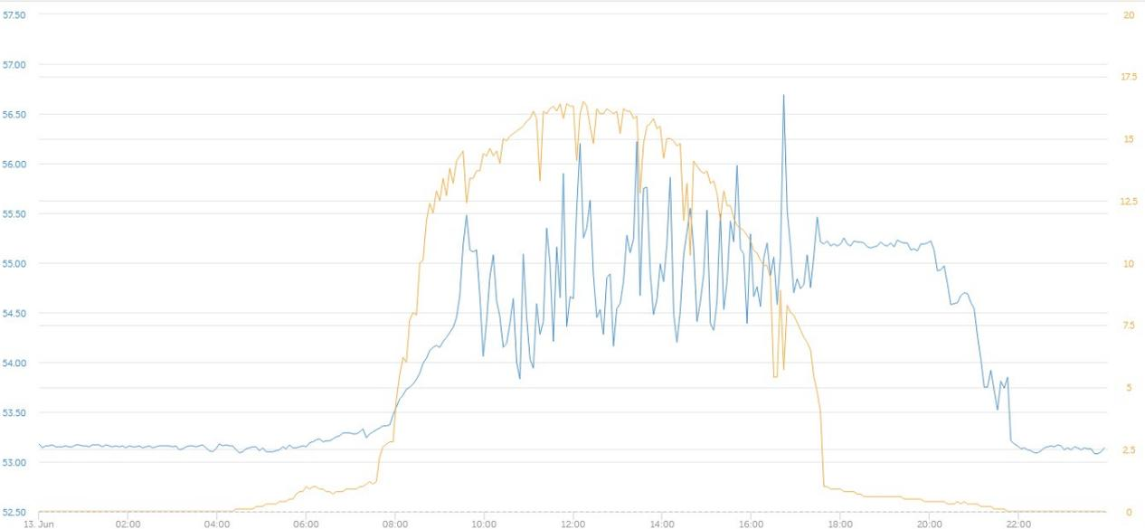
Solar Charger Battery Voltage and Current [278]
