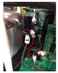
6. Check carefully that the converter PCBA has been installed correctly. Reconnect the AC and DC cables, replace covers and switch the unit on to test. Put the inverter or charger under maximum load to test the fan.
