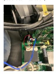
5. Mount the fan PWM converter PCBA with the supplied tie-wraps to the mounting eyes/holes of the fan. Connect the wire of the fan to the connection on the new fan control PCBA. Plug the connector of the new PWM converter PCBA to the original fan connector on the main board, as shown on the pictures below.
