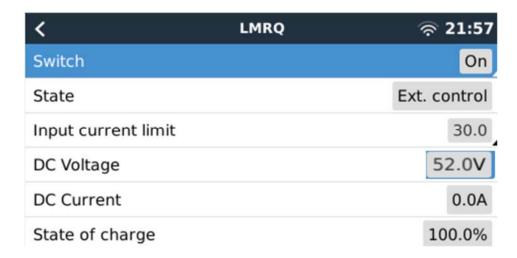
The Multiplus oscillate between « Bulk » and « Absorption » and never goes to « Float » mode. The charge voltage is now at 52V in less than 1 hour. The cells are well charged.
