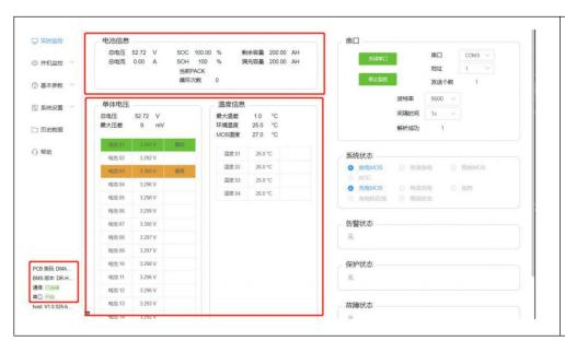
After the BMS communicates with the upper computer, you can monitor the basic parameters and status of the battery in real time. These information include battery voltage, current, SOC, SOH, cycle count, battery temperature, alarm status, protection status, etc.
