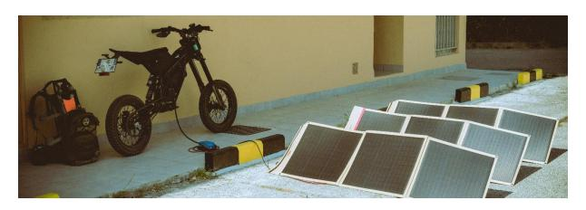
M.A.S.K (Mobile Autonomous Solar Kubie) has now apparently the World's First Portable 48V Direct Solar Charger of this type (not voltage "boosted" or "stepped down").
