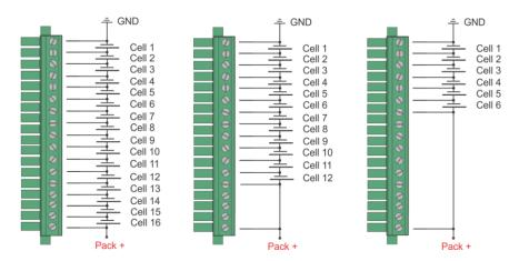
Figure 7: BMS unit power supply.
