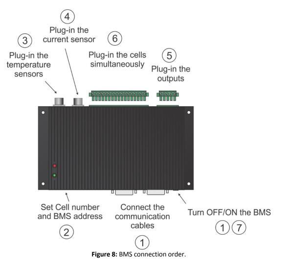
When disconnecting the unit from the battery pack, the procedure should be followed in reverse order.
