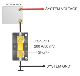
Figure 11: Shunt resistor connection.
