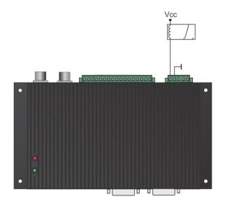
Figure 12: External signal relay with Vcc rated coil connection schematics.
