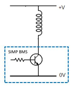
The principle of the gauges driver is identical to that of the grounding contactor control.
