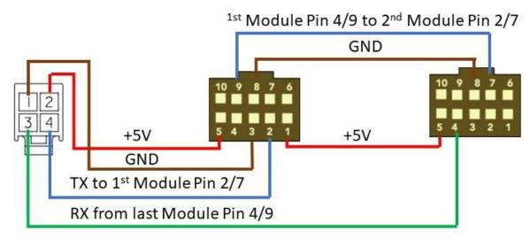
Connector 1 Tesla BMS Supplier Molex Family Mini fit 4 way Part no 39-28-x04x Harness Part 39-01-x04x
