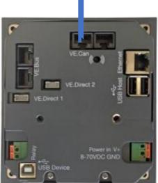
The GX control needs to be configured to 500kbps so it can receive the data from the SimpBMS.
