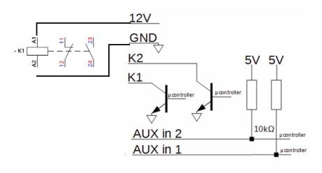
I can not use the connection below because there is a limit 100 mA for 12V pin. Is that correct?
