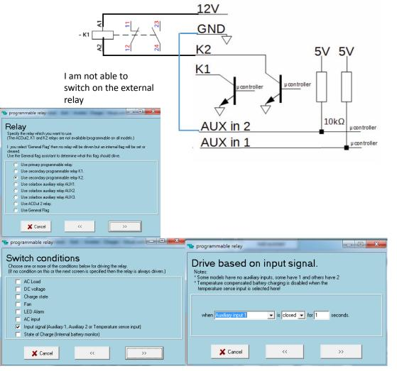
Relay K2 is ON when switch condition is "Auxiliary input 1" " open" . If I connect GND and AUX 1 nothing happens
